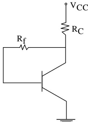
3. Find the small signal voltage gain in the following amplifier. Take  $\beta \gg 1$
