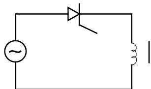
68. For the dc-dc converter shown, the peak SCR current is \_\_\_\_\_
